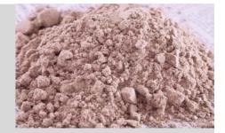
The thermoplastic resin was previously being dried in a V-cone tumble blender and transferred to trays for curing in an oven. Afterwards, the powders are milled to disperse agglomerates that have re-formed during curing. This three-step process took 24 hours to complete.
