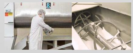
Shown is a Ross Ribbon Blender used for batching vitamin supplements and nutraceutical blends. In operation, ingredients are loaded into the blender, typically filling 40-100% of the rated capacity. This is up to the level of the outer ribbon's tip, leaving enough head space for the material to be vigorously agitated and mixed. Above photos show a batch during the discharge cycle.
